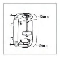
Step 3: Take out the weather-proof connector, separate it to four parts as screw nut, rubber ring, screw bolt and O-ring;
