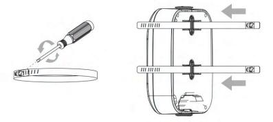
Step 3: Fix the rings with rear cover on the pole, fasten the screws;
